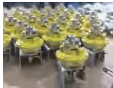
Kinetrol + Bronze head support (special design for customer)
